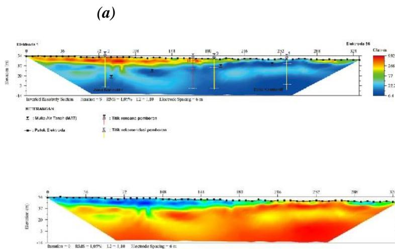
**Figure 3**(a) Conductivity cross section and (b) subsurface resistivity with groundwater drilling recommendations point on track 1
