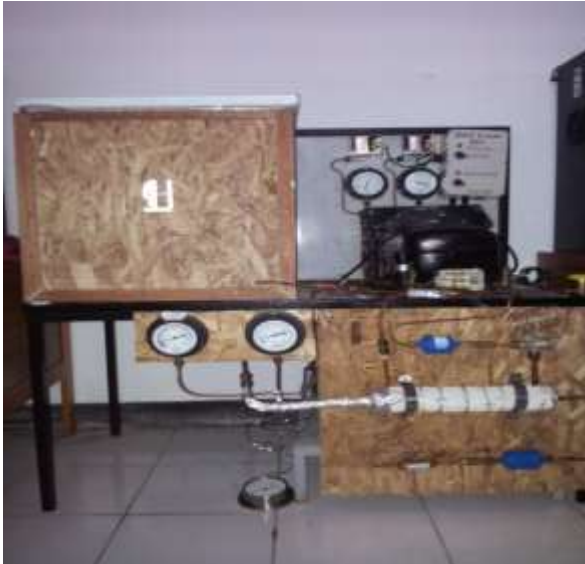
Gambar 4. Prototype mesin uji cascade
